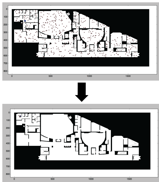
Figure 3: The first step and 10th step of the sequence. The robot was piloted towards the small room and the particles converged on its location.
