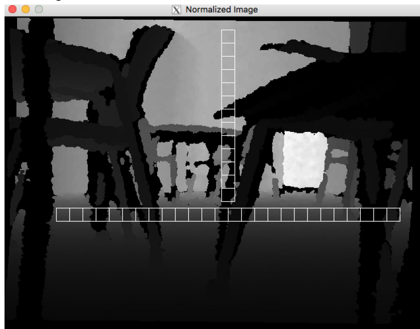
Figure 1: An example frame from our IR camera, with the iterable boxes spanning horizontally (and vertically, in this case). The darker objects are closer than the lighter objects.
